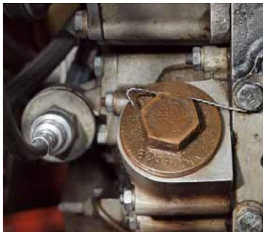
Oil screen cap on TCM engines without an oil filter. Note safety wire forming a reverse “S”, holding both ends tight.
