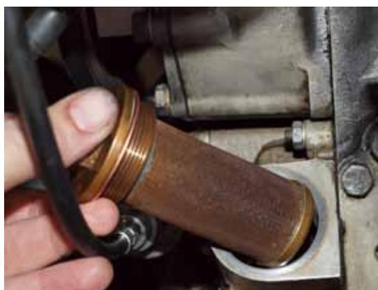
Removing TCM oil screen for cleaning
