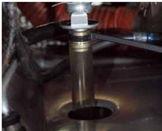
Oil quick drain valve with plastic drain hose attached
