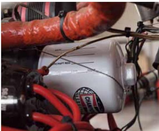
Oil filter installed on a Lycoming O-320 engine. Note attachment of safety wire.
